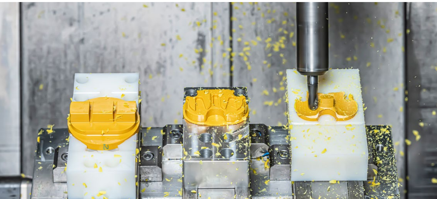
Test implants for knee joints: Machining on a machining centre in Cham.
