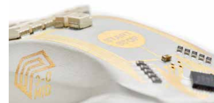
MIDster: Sample for a moulded interconnect device.
