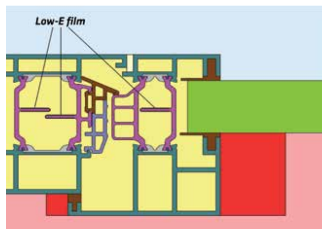
Uf = 1.7 W/m 2 *K: insulbar thermal insulation profile with Low-E film (marked in grey), ε = 0.03
