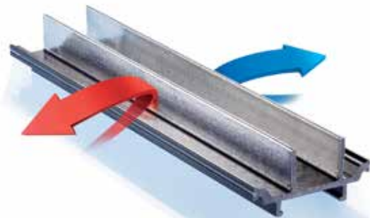
insulbar® LEF: The thermal insulation profile uses Low-E film which reflects thermal radiation. This provides an optimum thermal separation of the outside and inside shells of metal frames for windows, doors and facades.
