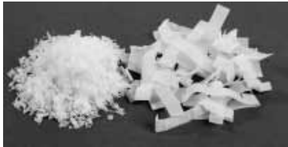
High degree of toughness prevents chipping and disruption during machining. Comparison of machining result between TECADUR PET (left) and TECAPET (right).
