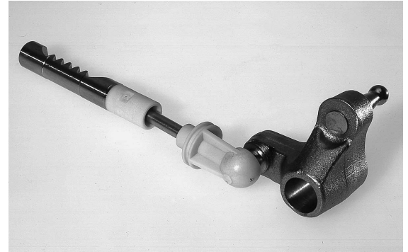
Rack for LuK: The two ball-and-socket joints made of TECAMID GF25 TF10mod. were cast directly on to the parts in a single production cycle by ENSINGER, using two-component technology.
